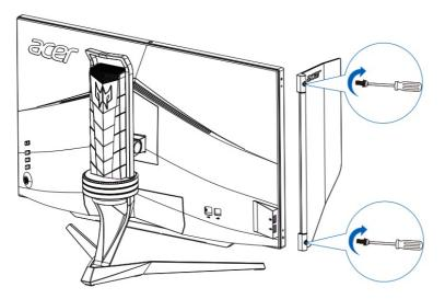
2. Use screwdriver or coin to fasten screw and fix door on the head.
