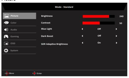
• Brightness: Adjust the brightness from 20 to 300.
