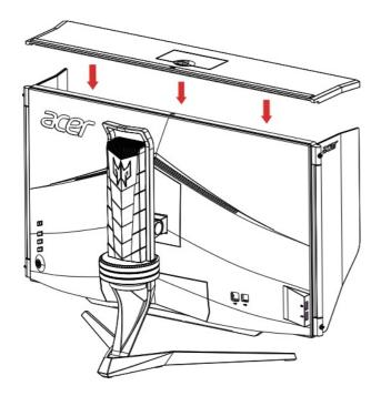
5. Shading hood installation complete.
