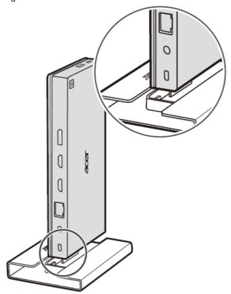
2. After the ridge is aligned, push the dock down into place.
