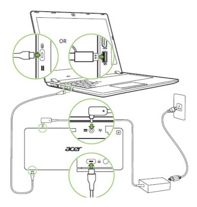
**Note:** When the dock is connect to the USB 3.0 on your notebook side, the functions of the dock may be limited. **Note:** When using the USB Type-C connector connecting to the dock, gently push it into the tunnel to the port. You will feel a click indicating it is connected.
