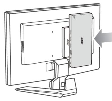
4. Make sure the hook is completely inserted into the slot.
