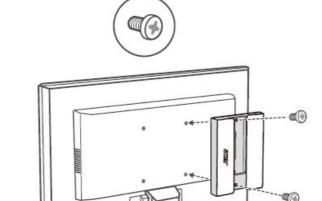
2. Hold the dock with the Acer logo facing you and the side with 2 ports facing up. Horizontally align the Acer logos on both sides. Align the hook on the left of the stand with the slot on the dock.
