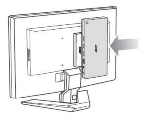
4. Make sure the hook is completely inserted into the slot.
