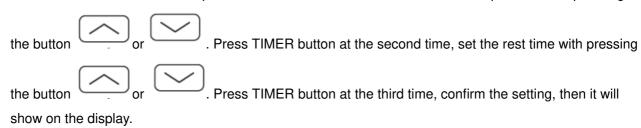
**Note:** It can be set to automatically turn off or on in 0.5-24 hours. Each press of the buttons will increase or decrease the timer. The Timer can be set in 0.5 hours increment below 10 hours and 1 hour increment for 10 hours or above. The SET light will turn on while setting. To cancel the set function, press the TIMER button again.
