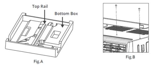
• NOTE: For safety reasons, all 4 screws must be used to attach the top rail.
