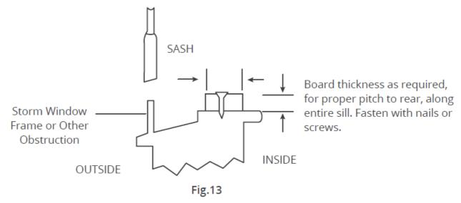
• If Storm Window Frame must remain, be sure the drain holes or slots are not caulked or painted shut.
