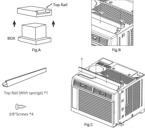
NOTE: For safety reasons, all 4 screws must be used to attach the top rail.
