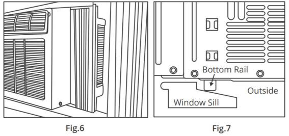
• Once the air conditioner is placed, extend both the left and right accordion panels to the width of the window.
