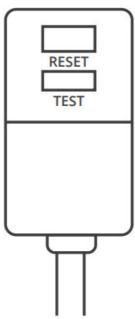
If a test is performed and the indicator light remains ON, the current leakage has been detected. Do not use the air conditioner or attempt to reset the LCDI Plug. Contact Customer Service for troubleshooting recommendations.
