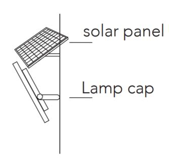
Make sure the solar panels are installed at the correct angle and they will not be blocked by the obstacles from the sunlight.
