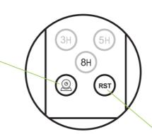
Reset: pressing over 5 seconds then you will hear "Dong-dong-dong" **6** the light source will flash twice in the meantime. It indicates the monitor has been reset successfully.
