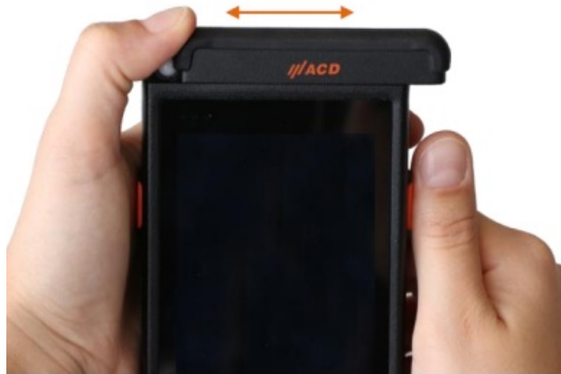
Figure 9: Attaching and removing the upper plug-in module
