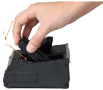
Figure 16: Inserting replacement rechargeable battery in the docking station
