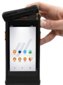
Figure 26: Removing the upper logistics protective cap
