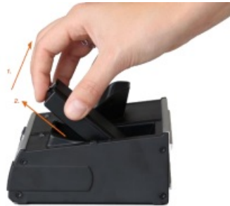
Figure 17: Removing replacement rechargeable battery from the docking station
