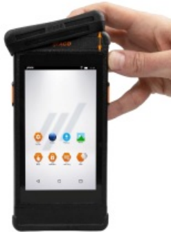
Figure 24: Attaching the upper logistics protective cap
