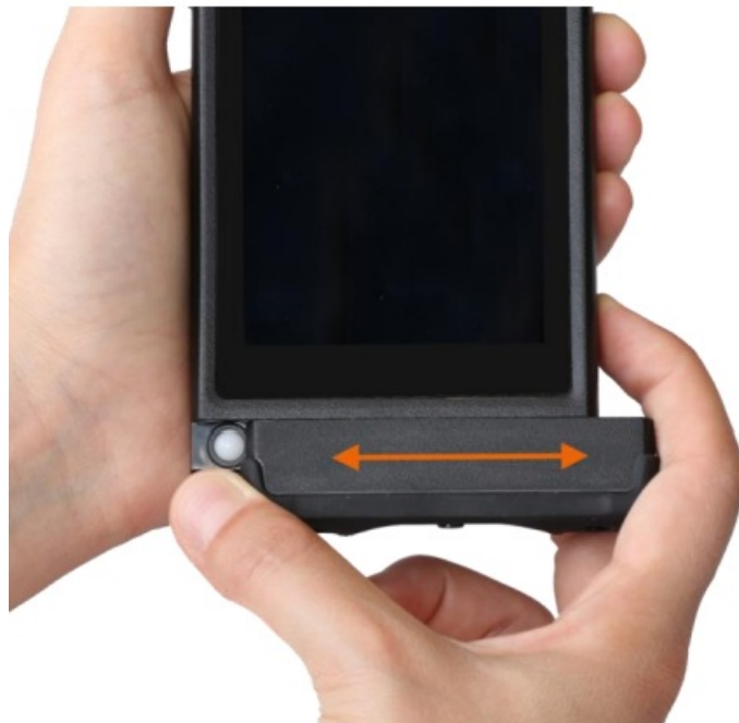
Figure 9: Attaching and removing the upper plug-in module
