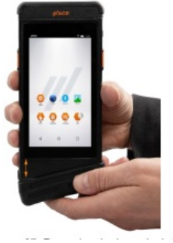
Figure 27: Removing the lower logistics protective cap
