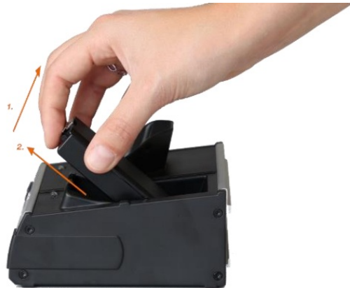
Figure 21: Removing replacement rechargeable battery in the docking station
