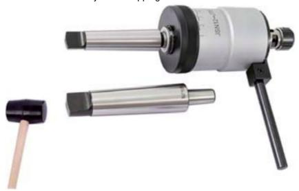
If the arbor has a taper, push and twist it into the tapping head, and then hit the end of the arbor with a mallet to fix it on the taper part of the tapping head. To remove the taper mount arbor, strike the side of the arbor several times with a mallet.
