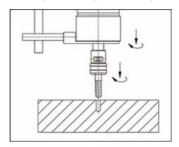
2. Start tapping by moving the machine spindle down with the chuck.
