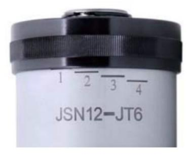
Set the clutch so that it would prevent the tap from breaking and ensure the tap can cut as needed into the work piece. You can choose a suitable torque level from numbers 1, 2, 3, 4 on the main body circumference based on the diameter and material of the work piece. The chuck can withstand different torque levels from low to high and can be adjusted by the TTT operator himself. For materials that are hard to tap, it is advisable to do two passes. JSN12-JT6
