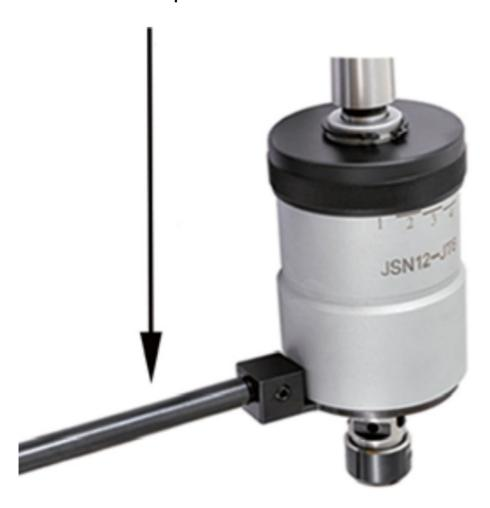
The stop arm needs to be rotated to reverse the direction of the tapping head.
