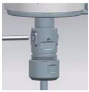
b. Insert the square end. of the tap handle into the square hole of the clamping device.
