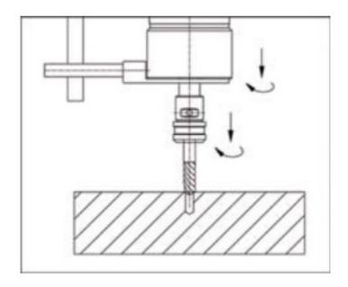
3. Stop the vertical movement of the machine spindle when it reaches the desired depth. The chuck spindle will keep tapping until it reaches the end of its extension, then it will automatically stop rotatin.
