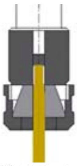
d. Tighten the lock nut with a wrench
