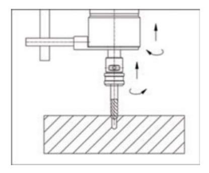
6. The tap will start rotating as soon as it has fully withdrawn from the workpiece.
