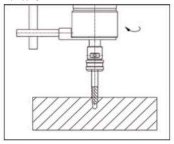
4. Lift the machine tool spindle. Then the chuck spindle and the tap will automatically rotate in reverse and quickly retract.
