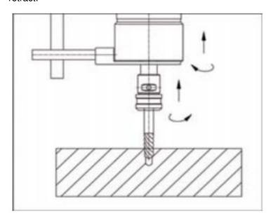
5. The raising speed of the machine spindle should match the retreating speed of the tap. Otherwise, the tap will stop and start intermittently
