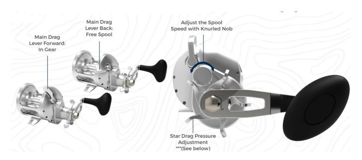
Adjusting the spool speed with knurl spool knob, you should tighten it all the way and put reel in free spool. Let the bait or lure hang off rod tip and slowly turn knob backwards until lure or bait slowly falls. This is a good setting to
