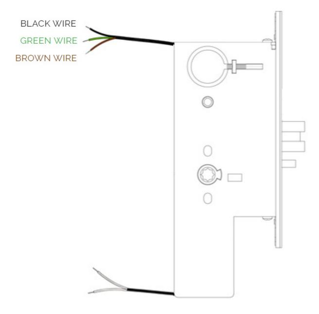
Two SPDT Mechanical Switches Mounted in Series Inside the Lockset
