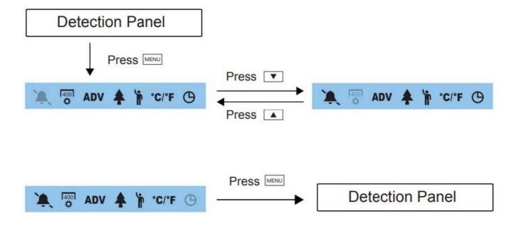
To set a particular function, press ENTER to enter this function when the icon is flashing, use arrow button to adjust the setting or figure, when it's done press ENTER to confirm and exit.
