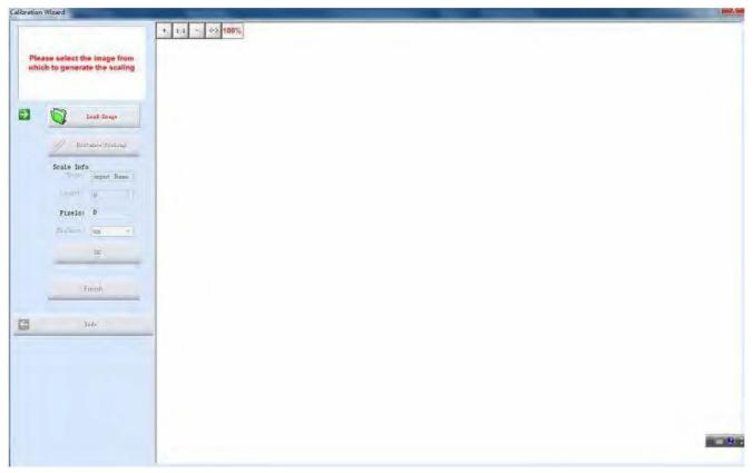
3. Click [Load Image] to load the calibration slide picture taken in Step1.
