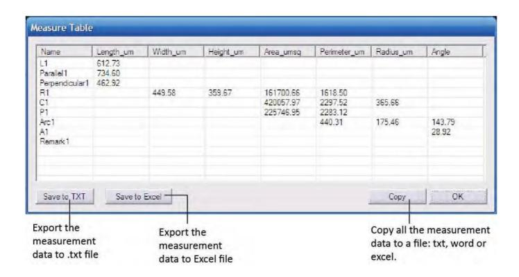
All the measurement data is listed in the [Measurement List]. The software allows you to export all the measurement data to TXT or Excel file.
