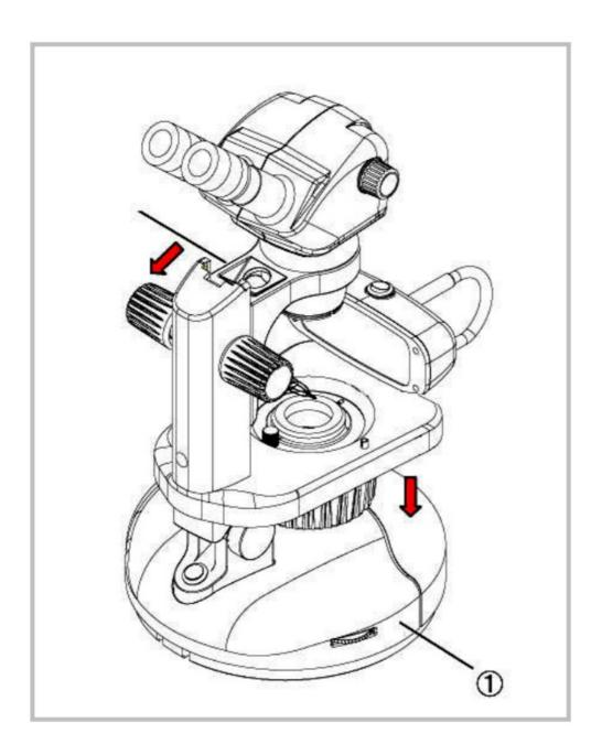
Rotate the Microscope to a suitable position for viewing comfort by gently pushing the base .
