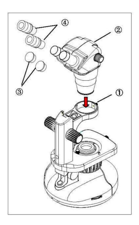
Loosen the lock screw on the stand and insert the stereo head into the bracket of the stand. Tighten the lock screw to secure the stereo head.
