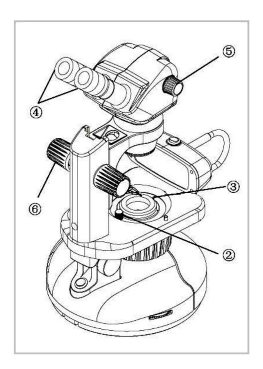
Close the baffle by turning the baffle control knob clockwise, and close the iris diaphragm by turning the iris diaphragm control lever clockwise.
