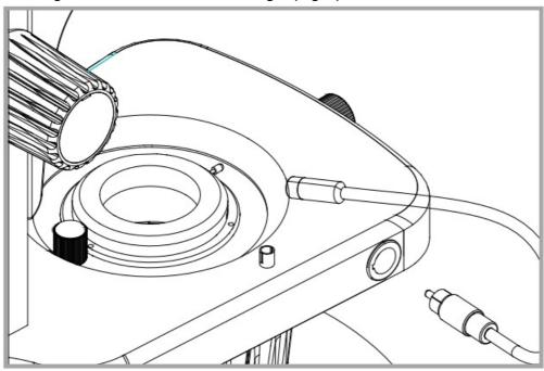
Connect the overhead fluorescent light to the front of the stage by lining up the male and female holes on the snap connector .
