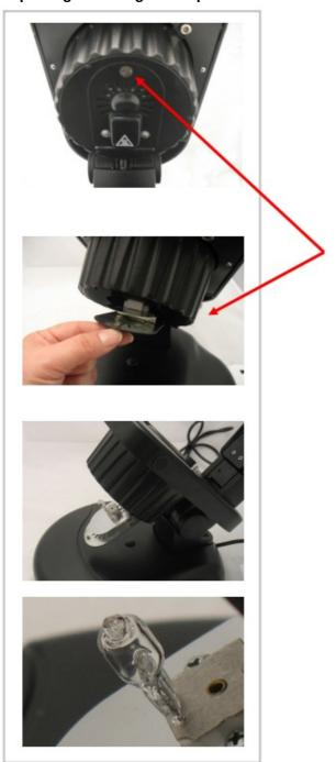
The darkfield illuminator (bottom light) uses one 6 volt, 20 watt tungsten halogen lamp – CAT #6047C.
