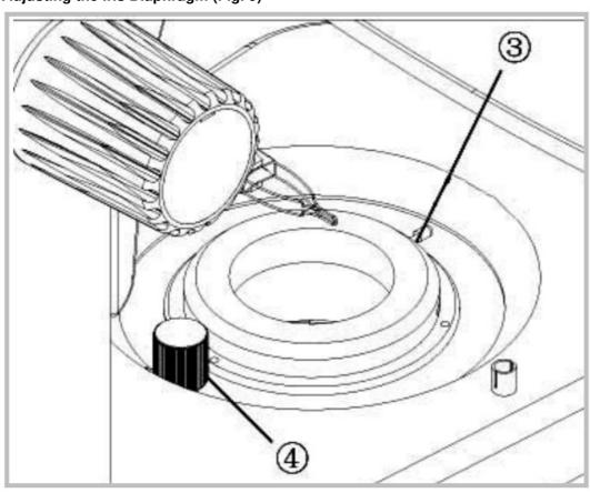
The iris diaphragm restricts the diameter of the beam of light entering the objective and therefore excludes
