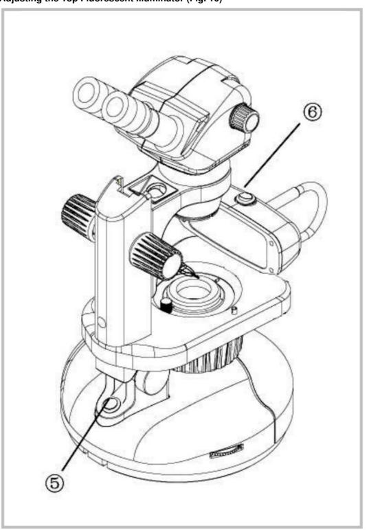
By turning the main switch to "I" (on) and the fluorescent lamp switch to "I" (on), the top illuminator will provide the equivalent of a northern daylight overhead light source.
