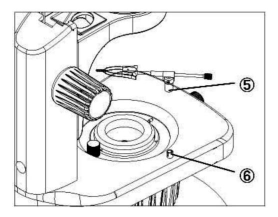
The stage has two stone holder mounts on either side of the stage where you can attach the stone holder
