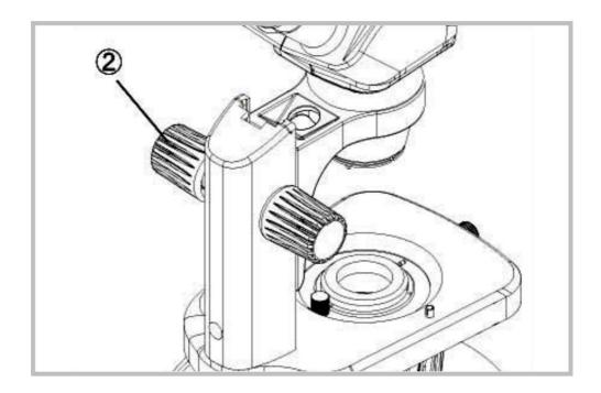
To adjust tension, hold both left and right focus adjustment knobs with both hands, hold the left knob (to prevent it from turning), and rotate the right knob clockwise to increase (tighten) or counterclockwise to decrease (loosen) the focus knob tension.
