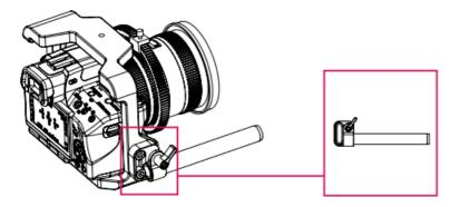
3. Controller mount adapter: If you need to mount the controller to the cage, you can use the screws to attach the adapter to the cage first, and then mount the controller to the adapter.
