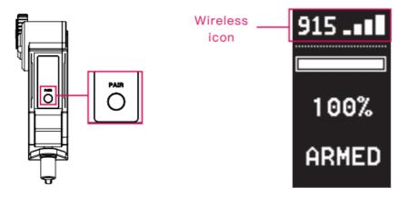
2 Hold the PAIR button on the controller until the wireless icon starts to flash on the controller's OLED screen;
