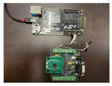
Simplicity Commander from Silicon Labs is used to flash the firmware onto the module.
