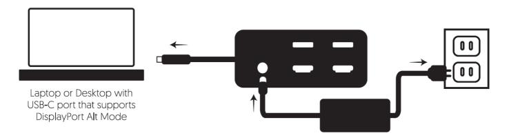
Connects up to 2 external displays, as needed, with HDMI cables [HDMI 2.0 cables for max resolutions].
