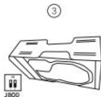
3.According to user needs to adjust the DIP switch, the factory setting is Double hard disk JBOD mode setting
