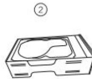
2.Align the HDD for installation Install the hard disk on the interface and fix it
