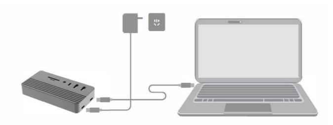
Connect PC port of hub to your PC with the accessary USB C to C data cable. Using large power consumption devices with hub, please plug a power adapter to PD port (60W-1 00W), otherwise the hub may work unstablly or does not work. For HDMI function, please ensure your laptop USB-C 3.1 Gen 2/USB-C 3.2/Thunderbolt 3 port supports DisplayPort Alt Mode.
