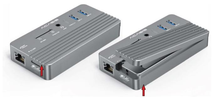
2. Stick the thermal pad onto the top of your SSD. At a 45° angle, slide in your SSD untill it is fully seated align with the edge.3
