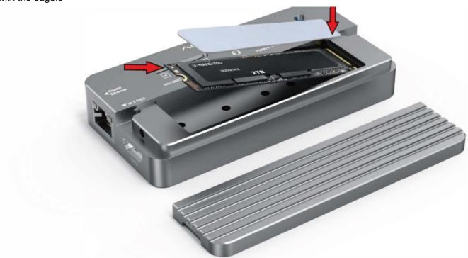
3. Fix SSD with the rubber grommet.
