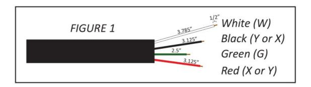
When making connections, make certain they are secure, properly insulated, and there are no stray wire strands outside the terminals. Tighten the terminal screws to 12-16 in-lbs torque. Tighten the cord clamp assembly screws to a maximum 10-12 in-lbs torque. Lastly tighten the assembly screws.
