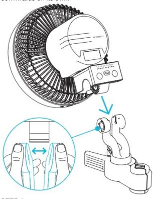
**STEP 3** Replace the knob of the mounting point as desired.
