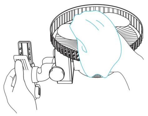
**STEP 5**Realign the grille over your clip fan, twist clockwise, then screw the grille back on to lock it in place.
