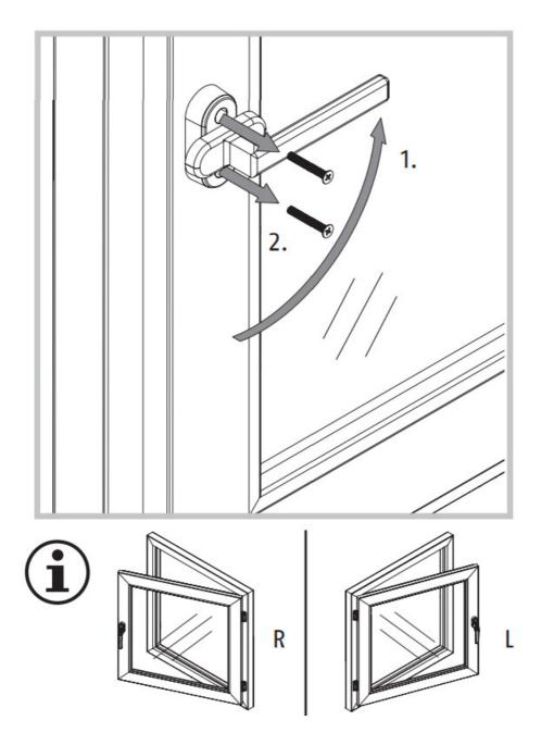
The instructions show the assembly on a right-hand window (R). The assembly is reversed for left-hand windows
