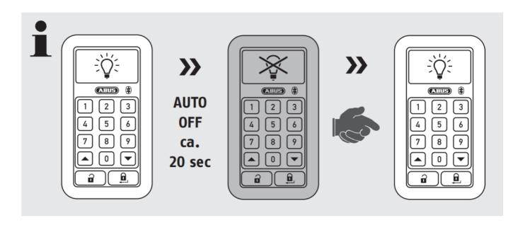
After approx. 20 seconds without any input, the display lighting goes off. To wake the keypad, tap the centre of the display firmly with your hand once.
