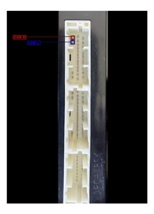
CB031 – Extension Cable for Direct Connecting to Toyota/Lexus Smart System with B9/BA Key – will let you make the connection to vehicles Toyota/Lexus equipped with Smart System with B9/BA Key. The connection to the smart system of the vehicle much easier, without the need to search for the CAN wires and puncture them. It helps in All Keys lost situation, when you need to read the Smart System Module.
