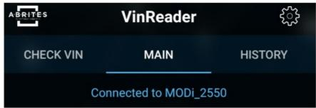
Once you connect the VIN reader to a power supply and your Bluetooth is ON you can select the VIN reader to connect to. You then select and your two devices are connected. Now you can start using the VIN reader.
