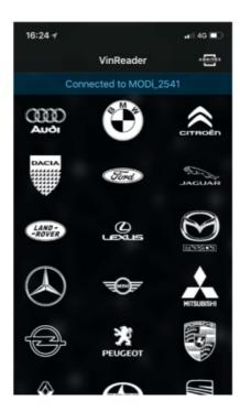
Select the brand you are about to work with and the VIN reader will start scanning the VIN numbers of the electronic modules installed in the car.
