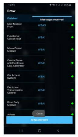
In green, you will see a VIN number when it is correct as per the rest of the modules in the vehicle and in red you will see the modules which do not match the rest of the modules. Here is the screen you see while scanning the vehicle and the discovered units and their amount. You will start seeing the response from the electronic modules straight away. Here is an example where the modules are scanned and there is no problem determined by the VIN reader.
