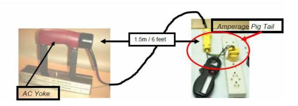
The Amperage Pig Tail is a short length of power cord (18-3), that has a Male Plug installed on one end and a Female Plug installed on the other end (Illustrated above). After the Plugs are connected, and the clamp type
