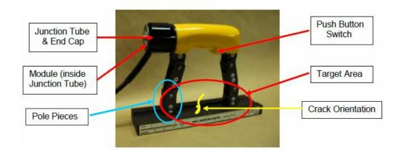
Solid State Push Button Switch – The Solid State Push Button Switch was designed for comfort and safety.
