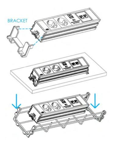
OPTION 1 - Fix the module onto a flat surface
