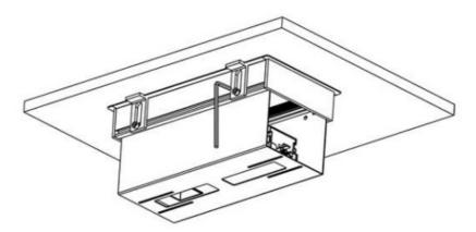
4. Tighten the screws using Allen key.
