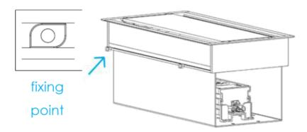
3. Place the L tighteners onto the fixing points.
