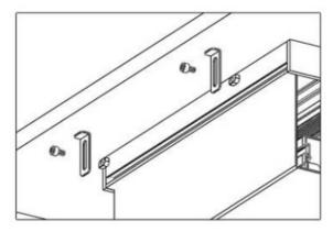
2. Place the fixing point into the sliding cannol.
