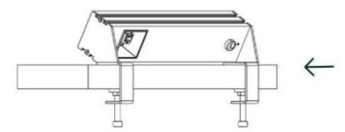
2. Use Allen key to fixate the module onto the desk
