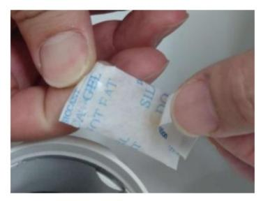
Stick a double-sided tape on desiccant bag. Pull the adhesive tape cover in order to attach the desiccant bag to the camera.
