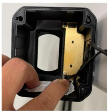
Put back the cover of the camera as soon as the bag is replaced. (If you leave it open too long, the desiccant bag will start absorbing water from the environment.) **Step7.** Be sure the cover is closed tightly.
