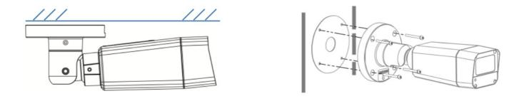
**Step 4:** Loosen the three hex socket bolts and adjust the camera to the required angle. Then re-tighten the screws, and adjust the position of the sunshield.
