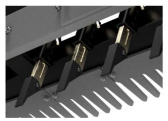
3. **Step 3:** Remove the ½" bent pins from the upright mast on the back that is locking down the leveling blade. If these pins are already up then skip this step and move on to step 4. If the pins are in place and cannot be removed from the uprights, then the TR3 may need to be lowered to the ground to take the pressure off the pins. Remove the pins and pin each one in the top hole on the uprights.
