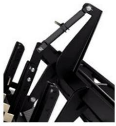
The ratcheting top link bracket may need to be extended to allow the bracket to be secured to the TR3. Use the center handle on the ratcheting top link to extend out the top link until the bracket is able to be secured the to center top mast on the TR3.
