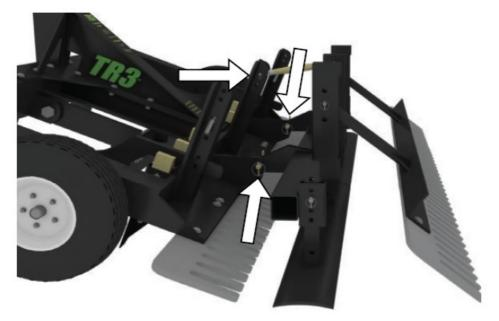
2. **Step 2:** With the TR3 in base position (covered above in TR3 setup, with Scarifiers lifted out of play) and the Profile blade lifted up so that is out of play; adjust the TR3 so that the Finish Rake attached to the TR3 is roughly 3/4" to 1" off the ground. This will allow material to properly flow through the TR3, and back to the Profiler attachment.
