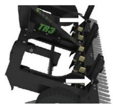
4. **Step 4:** Make sure the Stabilizing wheels are mounted in the middle hole on the tire mounted bracket. This can be adjusted later if needed. For now make sure the tire is mounted in the center hole.
