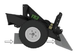
**NOTE**: Due to 3 point hook ups on some models of tractors, it may be necessary to move the tires on the TR3 forward or back a hole to properly adjust the TR3. If you are not able to adjust the TR3 so that the Leveling Blade and Finish Rake touch at the same time try moving the wheel forward one hole and then repeat Step 5.
