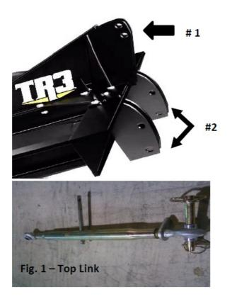
**Step 1** – Attach the tractor to the lower arms indicated by arrow #1 in the picture. There are two connecting holes on the TR3 for the bottom arms of the tractor to attach to. If the TR3 is connected to the bottom holes, then make sure to connect the Top Link in the bottom holes on the mast shown by the arrow labeled #2. If the lower arms of the tractor are connected to the TR3 in the top hole, connect the Top Link using the top hole as well. The Top Link is shown in Fig. 1.
