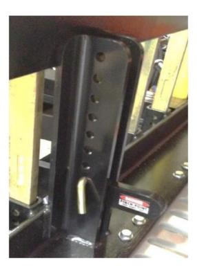
**Step 3** – Make sure the Stabilizing wheels are mounted in the middle hole on the tire mounting bracket. This can be adjusted later if needed. For now make sure the tire is mounted in the center hole.
