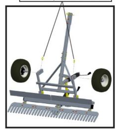
Remove nut,washers, spacers (if supplied) and bolt.
