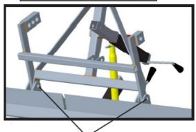
While one person is holding the Tongue and Body Frame, the other person holds the Wheel Axle assembly while pulling the bolts out.
