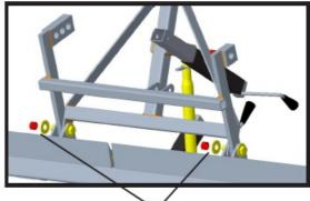
Remove washers and nuts (leave bolts in place).
