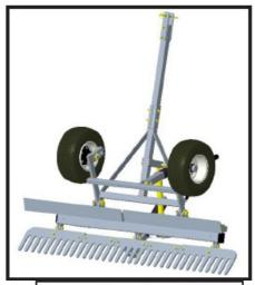
Remove Lynch Pins and slide both wheel/hub assemblies off.
