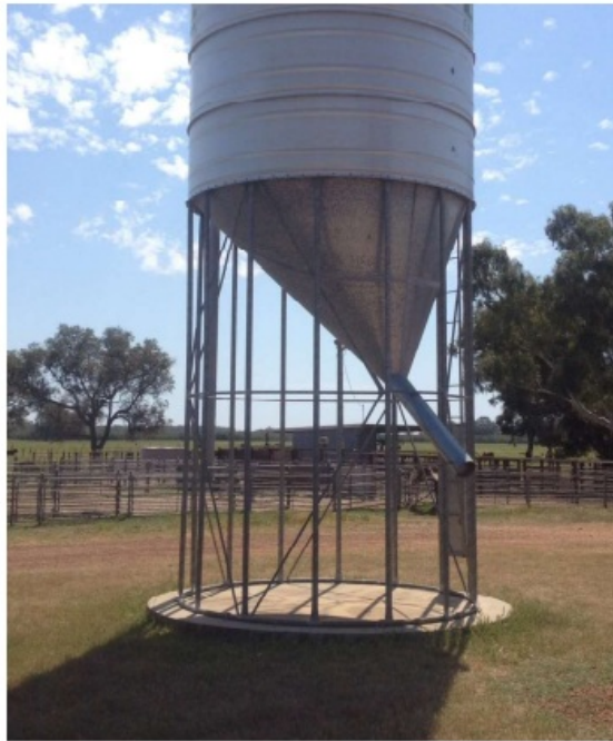
Figure 3: Example of silo with an asymmetric cone
