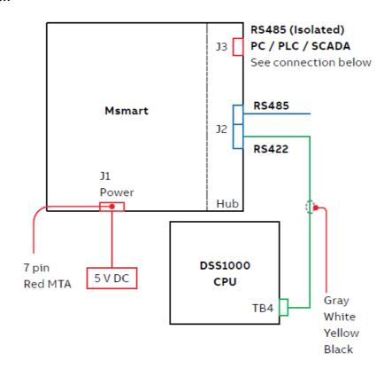
Msmart connection diagram to MVC4 medium voltage soft starter.
