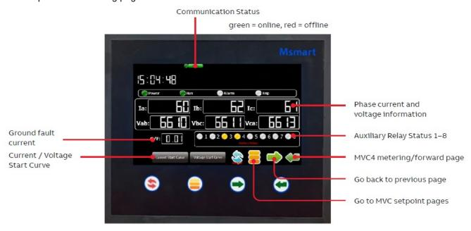
The MVC4 setpoint pages can be accessed by pressing the button. See chapter <MVNAME> programming for more information. The MVC4 metering pages can be accessed by pressing the button. See chapter <MVNAME> metering for more information.
