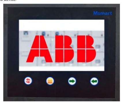
Msmart consists of a touchscreen and four membrane buttons for navigation that can be used when the system is installed in a harsh environment.
