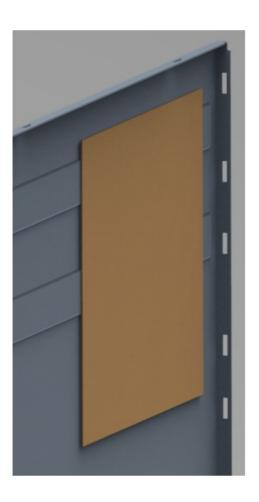
When mounting on an aluminum attachment profile or the wooden mounting plate use the screws which come fixed to the metering plate.
