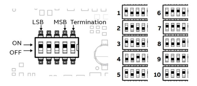
The address must be between 1 and the maximum number of FusionAir devices supported by the controller to which it is connected:
