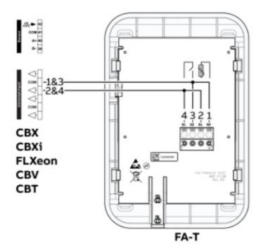
Alternatively, they can be connected to a single analog input, and logic in the Controller Strategy can derive the switch position. The digital input is a push-button on the side of the FusionAir device and can be used for example to over-ride a schedule for 1hr or override until the next value change.
