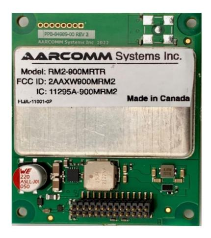
This information should be referenced when designing the host interface PCB to the RM2-900 MRTR. The AARCOMM model RM2-900MRTR is a frequency hopping spread spectrum (FSS) transceiver module designed to be compatible with U.S. (FCC Part 15.247) and Canadian (RSS-210) regulations for license free use in the 902-928 MHz ISM band.
