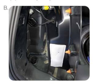
STEP 4: Locate the vehicle's Green/Brown (A.) wire that is located in the harness above the rear passenger wheel well (B.)
