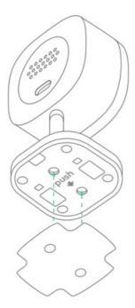
b) Remove another side film of 3M tape and stick the device to the wall, rotate the camera to the position you want to see.
