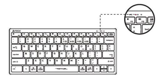
The flashing Red light indicates when the battery is below 10%.
