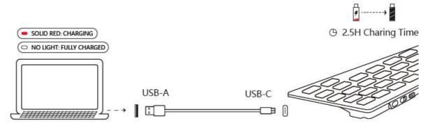
Bulit-in 300mAh rechargeable lithium battery, it can be used for up to 3~5 months when fully charged.
