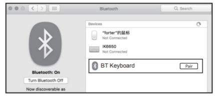
3. Bluetooth searches for "BT Keyboard" and clicks "Pair" to complete the installation and it can be used properly
