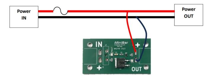
NOTE: Red Fault LED will not operate when crowbar trips.
