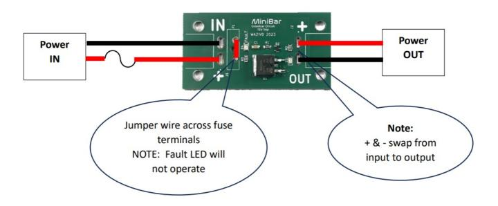
**NOTE:** Max of 15 Amps Continuous or 25 Amps @ 50% or less duty cycle (30 seconds) Maximum fuse size: 30 Amps
