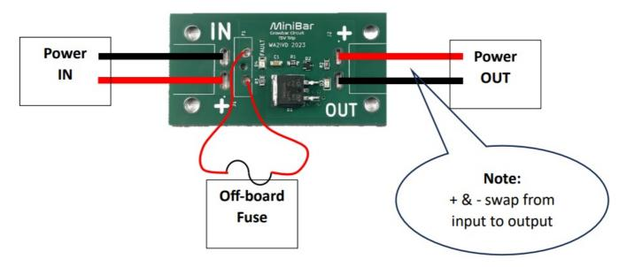
**NOTE:** Max of 15 Amps Continuous or 25 Amps @ 50% or less duty cycle (30 seconds) Maximum fuse size: 30 Amps
