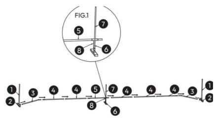
**STEP 4:** Slide the net over one of the #1 pipes in the half, then half of the #7 pipe, and then half of the other #1 pipe. Lastly, slide the whole net to the bottom gradually.
