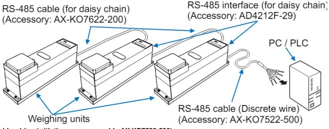
• Cable wiring (with the accessory cable AX-KO7522-500)
