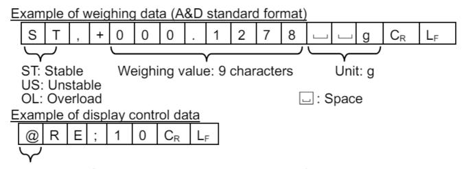
Data with "@" at the beginning is control data for when a display unit is connected. Ignore this data during communication with a PLC via RS-232C.
