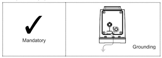
Wire the power line and signal line to ensure distance from power supplies for driving equipment and other lines that carry large currents.
