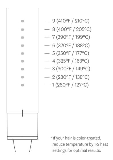
1. To power on, turn the SmartTwist dial once to the right. Lights will cascade, then turn solid when the tool is ready to use.
