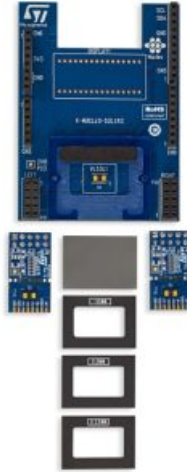
Figure 1. X-NUCLEO-53L1A2 expansion board, spacers, cover glass, and breakout boards
