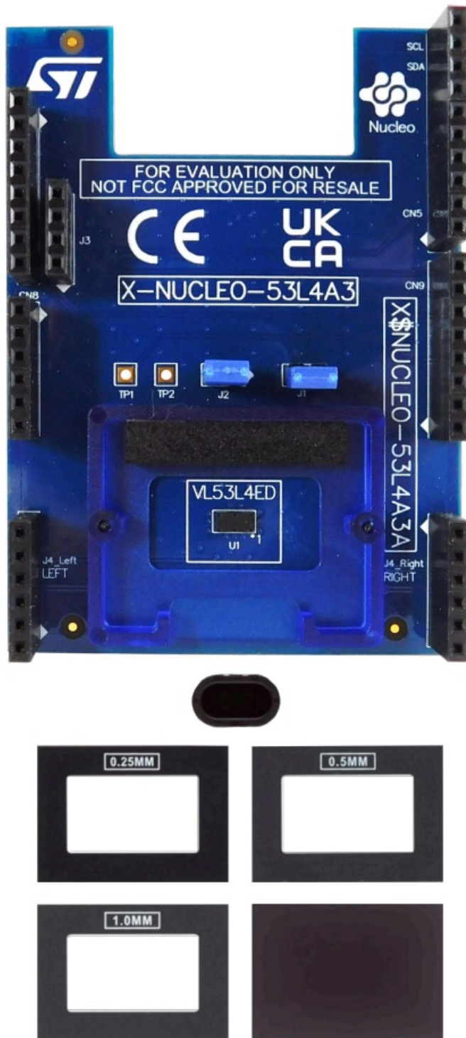
Figure 1. X-NUCLEO-53L4A3 expansion board, spacers, cover glass holder, and oval cover glass
