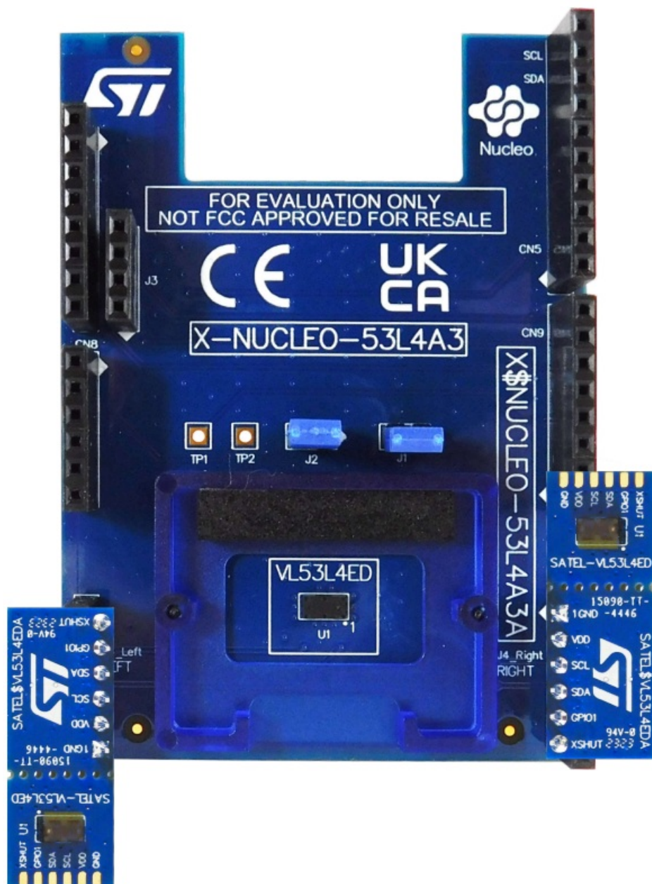
Figure 7. VL53L4ED mini PCB flying wire connection to the X-NUCLEO-53L4A3 expansion board
