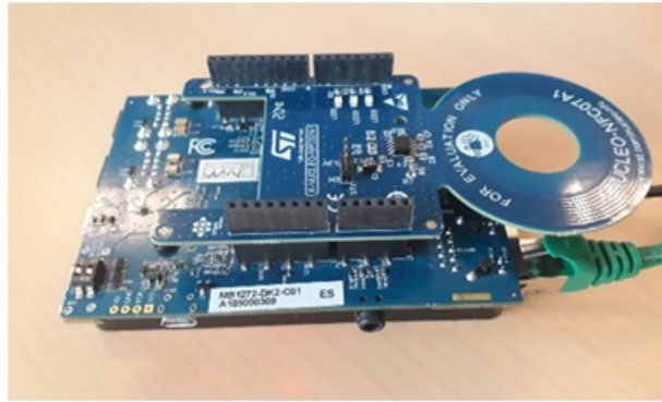
Figure 3. Full hardware connection setup
