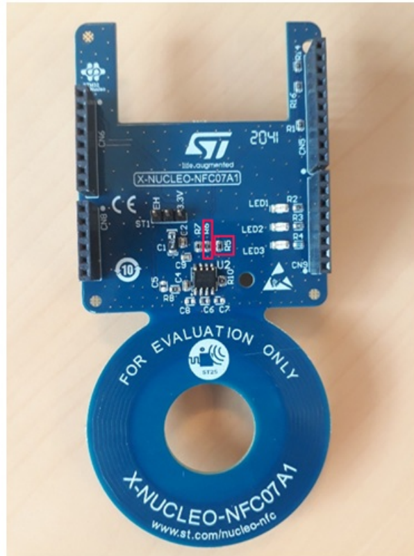
Figure 1. X-NUCLEO-NFC07A1 pull up resistors
