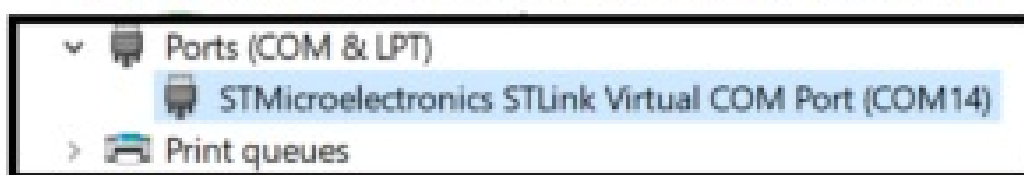
Figure 6. Screenshot of device manager showing virtual com port
